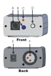
The PX-RGB dongle operates on 916 MHz and has a communication range of +400 feet line of sight is not required. 916 MHz a frequency not commonly used so wireless devices such as microphones and speakers will not interfere with the operation. The 916 MHz frequency is well below the 2.4GHz widely used by other wireless LED manufacturers.
