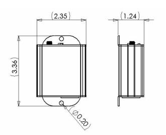
Frequency: 916 MHz Power supply: 9-12 volts 2.5mm power jack Max current: 150ma
